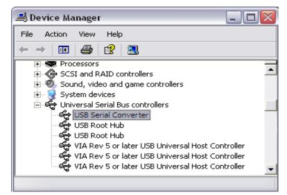
**1.4) Installation -** If the installation is not done correctly, it means the USB device is displayed with a question mark, then start the installation manually over the selection of *Properties -> Update Driver* or using the *Control Panel -> Add Hardware*. It will appear the *New Hardware Wizard*.
