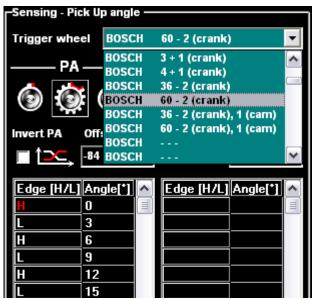
**2.3)** Rotation sensor - MASTER unit supports all known types of sensors and automatically adjust the sensing voltage levels, according to entered sensor type. The voltage levels can be also manually tuned as needed.
