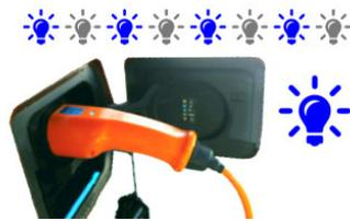
After connecting to the car, the blue LED flashes to indicate that charging is in progress.
