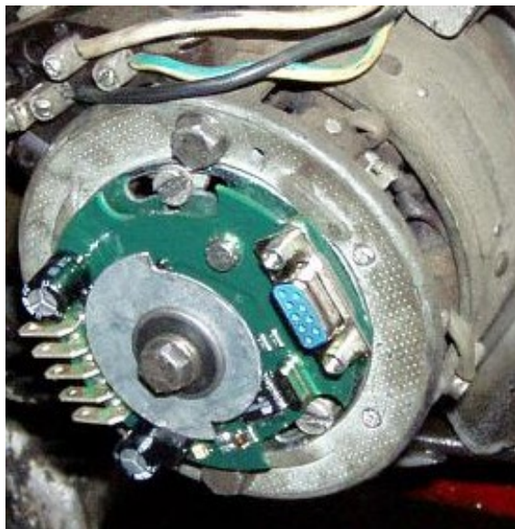
3. Screwing the shading sheet metal set to 28° advance (26-30° according to engine type)
